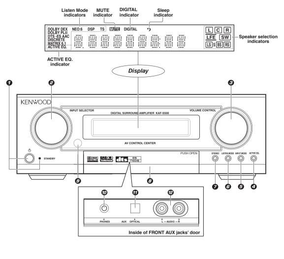
O ⊕ (POWER) key Use to turn the main power on or off. + 15 STANDBY indicator Lights when stand by mode. **Ø INPUT SELECTOR knob** + 18 (DVD/CD, VIDEO 1, VIDEO 2, FRONT AUX) Use to select input sources. O VOLUME CONTROL knob + 18 ACTIVE EQ key + 19 Use to select ACTIVE EQ's setting. INPUT MODE key + 9 Use to switch between the full auto, digital and analog inputs. **G** LISTEN MODE key + 23 Use to select the listening mode.
